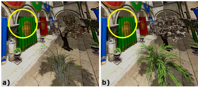
Figure 10: Two images from Patney et al.’s [2016] foveated renderer. In both images, the viewer is gazing towards the green curtain (noted by the yellow circle) and regions outside the circle are rendered at progressively coarser resolution. Low resolution shading uses coarser mipmap levels, causing most alpha tests to fail using (a) traditional alpha testing. With (b) hashed alpha testing, the foliage maintains its aggregate appearance.
