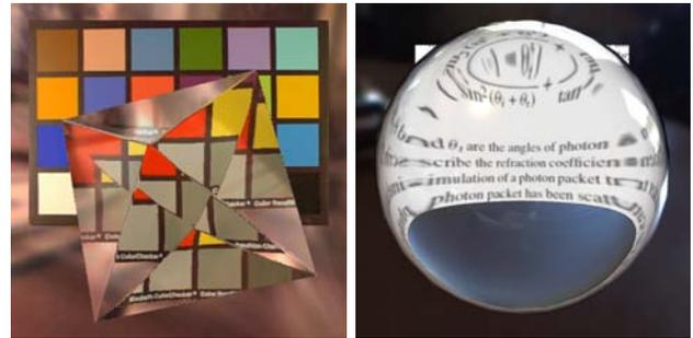
Figure 14: Errors arising in image-space refraction. (Left) Incorrect handling of total internal reflection. (Right) Aliasing problems become more noticeable as  $\vec{T}_2$  diverges further from the view vector. In the sphere, aliasing becomes visible near the silhouettes.
