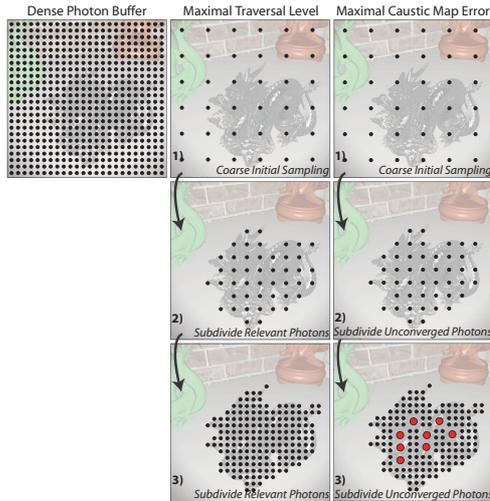
**Figure 5:** Compare previous dense photon sampling with adaptive sampling using our proposed metrics. For the maximal traversal level, relevant photons are subdivided until reaching some finest subdivision level. The maximal caustic map error subdivides relevant photons unless the children converge, when a single photon cluster is emitted. Photon clusters are not considered during further subdivisions.
