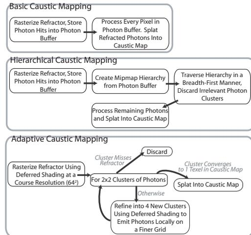
**Figure 6:** A high-level comparison of caustic map creation via basic, hierarchical, and adaptive caustic mapping.
