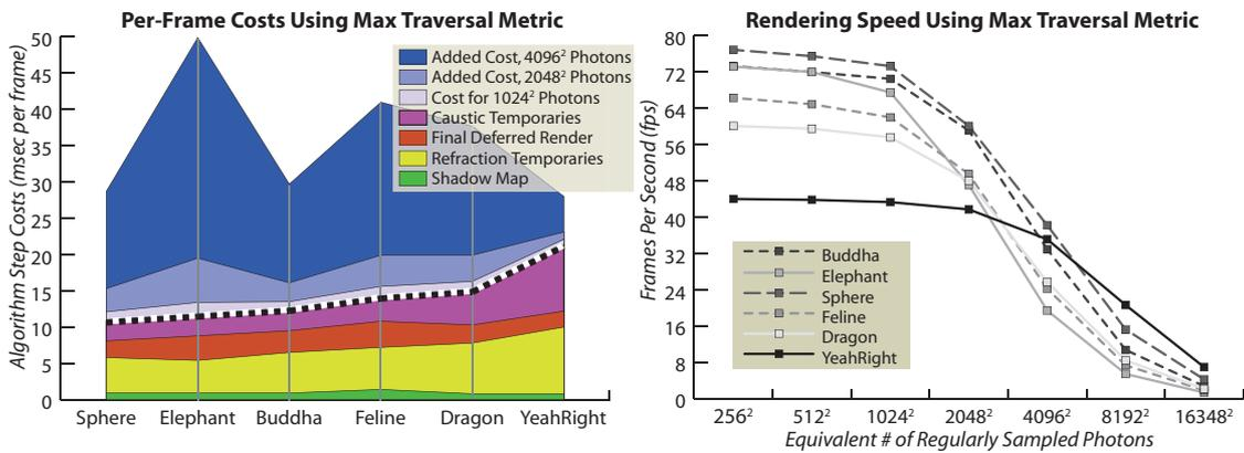
**Figure 11:** The left chart breaks out per-frame costs of individual steps in our adaptive algorithm using the maximal traversal metric. Steps below the thick dashed line are fixed, no matter how many photons are adaptively generated. Costs reported using  $4096^2$  and  $2048^2$  photons are the incremental costs beyond the next coarsest sampling. The right graph demonstrates how final framerates for our scenes vary with changes to the maximal traversal level.
