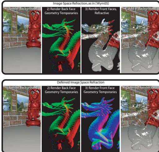
**Figure 3:** Compare image-space refraction and our deferred rendering approach. One key difference is that steps 2 and 3 for deferred rendering can be combined, touching refractor geometry to output front and back faces just once.
