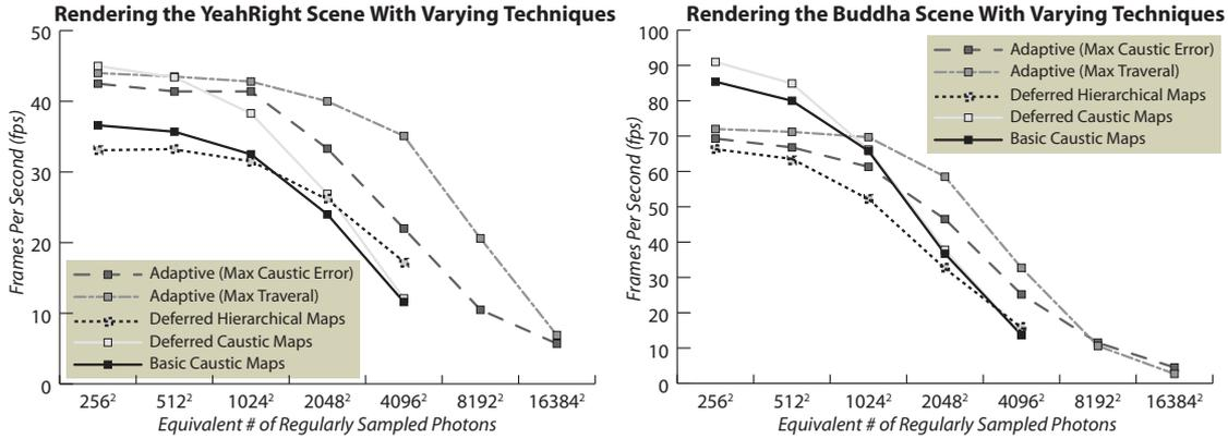
**Figure 10:** Variations in rendering speed using five different caustic mapping techniques: simple caustic maps [WD06], deferred caustic maps (i.e., a dense photon buffer with a deferred render pass), deferred hierarchical caustic maps (based upon [Wym08]), and adaptive caustic maps using the maximal traversal and maximal caustic map error metrics.
