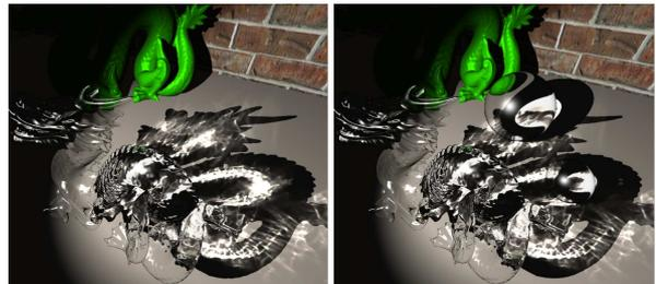
**Figure 13:** Caustics from a refractive dragon. (Left) With just the dragon the scene runs at 35 fps. (Right) Adding two occluded spheres slows rendering to 34 fps.
