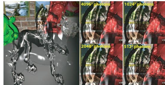
**Figure 1:** Adaptively computed caustics from a 100k triangle feline model. Our results allow dynamic lighting, viewpoint, and geometry at 24 fps for quality equivalent to a  $4096^2$  regularly sampled photon grid. Lower quality results, for  $2048^2$ ,  $1024^2$ , and  $512^2$  photon grids run at 50, 62, and 65 fps. The insets show varying quality settings.
