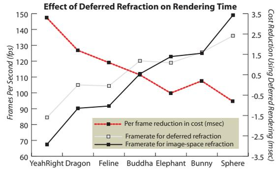
**Figure 9:** Graph comparing costs of previous image-space refraction and deferred shading. Performance on low-polygon models actually degrades, as repeatedly rendering these models costs less than the overhead to defer shading.
