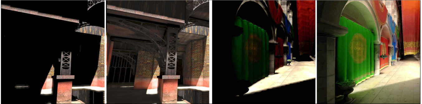
Figure 1: Direct-only vs. both direct and indirect in two systems. Cloud indirect computed and encoded in (left two) lightmaps and (right two) voxels. Please see the video for dynamic lighting.
