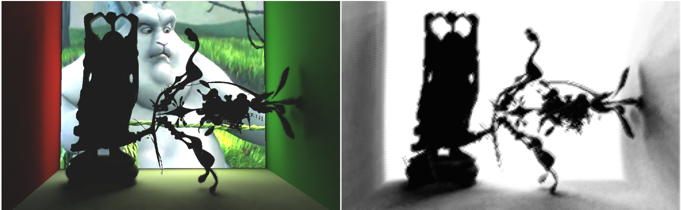
Figure 1: A simple scene illuminated solely by a large area light source displaying a video; (left) with illumination; (right) visibility only. Illumination varies in real-time as the video plays, and the complex soft shadows change convincingly as the objects are manipulated.
